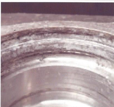
A nice new seal groove (top) and an oxide corroded one. Time for a caliper rebuild if yours looks like the bottom one.
